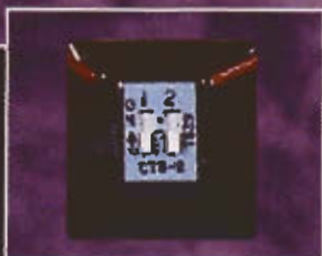
Get inside to tweak your tone. On-board preamp features a dip switch for adjusting the center frequency of the mid-range to 250, 500, 700, or 850 Hz.
